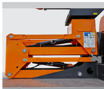
Hydraulic lift elevator (3 m)
