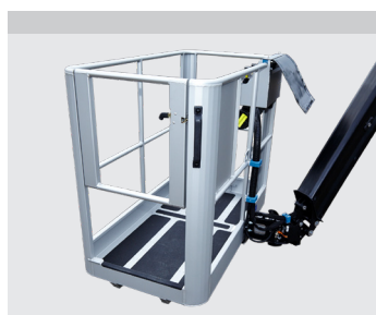
6 cm ground clearance below the end mounted aluminium basket
